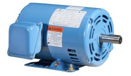
IronHorse MTDP premium efficiency AC induction motor, general purpose and inverter rated, 1hp, 3-phase, 208-230/460 VAC, 1800rpm, ODP, NEMA 143T frame, rolled steel, rigid base mount.
