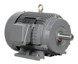
IronHorse MTCP2 premium efficiency AC induction motor, general purpose, inverter rated and severe duty, 7-1/2hp, 3-phase, 230/460 VAC, suitable for 208 VAC at 60 Hz, 3600rpm, TEFC, NEMA 213T frame, cast iron, rigid base mount.
