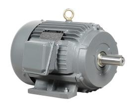
IronHorse MTCP2 premium efficiency AC induction motor, general purpose, inverter rated and severe duty, 7-1/2hp, 3-phase, 230/460 VAC, suitable for 208 VAC at 60 Hz, 1800rpm, TEFC, NEMA 213T frame, cast iron, rigid base mount.
