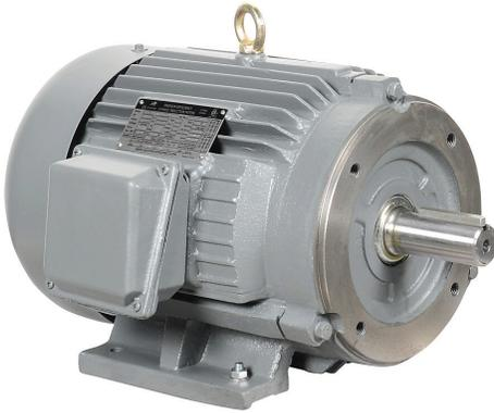
IronHorse MTCP2 premium efficiency AC induction motor, general purpose, inverter rated and severe duty, 7-1/2hp, 3-phase, 230/460 VAC, suitable for 208 VAC at 60 Hz, 1800rpm, TEFC, NEMA 213TC frame, cast iron, C-face/rigid base mount.
