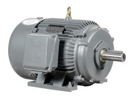
IronHorse MTCP2 premium efficiency AC induction motor, general purpose, inverter rated and severe duty, 7-1/2hp, 3-phase, 230/460 VAC, suitable for 208 VAC at 60 Hz, 1200rpm, TEFC, NEMA 254T frame, cast iron, rigid base mount.
