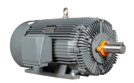
IronHorse MTCP2 premium efficiency AC induction motor, general purpose, inverter rated and hazardous location, 300hp, 3-phase, 460 VAC, 1800rpm, TEFC, 449T frame, cast iron, rigid base mount.
