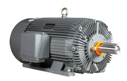
IronHorse MTCP2 premium efficiency AC induction motor, general purpose, inverter rated and severe duty, 250hp, 3-phase, 460 VAC, 1800rpm, TEFC, NEMA 449T frame, cast iron, rigid base mount.
