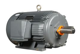
IronHorse MTCP2 premium efficiency AC induction motor, general purpose, inverter rated and severe duty, 200hp, 3-phase, 230/460 VAC, suitable for 208 VAC at 60 Hz, 1800rpm, TEFC, NEMA 445/7T frame, cast iron, rigid base mount.
