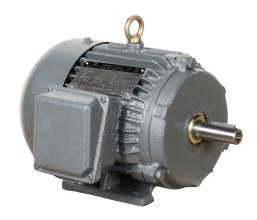
IronHorse MTCP2 premium efficiency AC induction motor, general purpose, inverter rated and severe duty, 1-1/2hp, 3-phase, 230/460 VAC, suitable for 208 VAC at 60 Hz, 3600rpm, TEFC, NEMA 143T frame, cast iron, rigid base mount.
