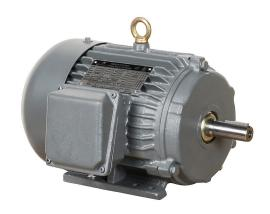
IronHorse MTCP2 premium efficiency AC induction motor, general purpose, inverter rated and severe duty, 1-1/2hp, 3-phase, 230/460 VAC, suitable for 208 VAC at 60 Hz, 1800rpm, TEFC, NEMA 145T frame, cast iron, rigid base mount.
