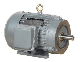
IronHorse MTCP2 premium efficiency AC induction motor, general purpose, inverter rated and severe duty, 1-1/2hp, 3-phase, 230/460 VAC, suitable for 208 VAC at 60 Hz, 1800rpm, TEFC, NEMA 145TC frame, cast iron, C-face/rigid base mount.
