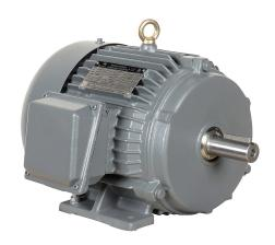
IronHorse MTCP2 premium efficiency AC induction motor, general purpose, inverter rated and severe duty, 1-1/2hp, 3-phase, 230/460 VAC, suitable for 208 VAC at 60 Hz, 1200rpm, TEFC, NEMA 182T frame, cast iron, rigid base mount.
