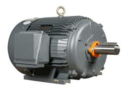
IronHorse MTCP2 premium efficiency AC induction motor, general purpose, inverter rated and severe duty, 150hp, 3-phase, 230/460 VAC, suitable for 208 VAC at 60 Hz, 1800rpm, TEFC, NEMA 445T frame, cast iron, rigid base mount.
