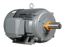
IronHorse MTCP2 premium efficiency AC induction motor, general purpose, inverter rated and severe duty, 125hp, 3-phase, 230/460 VAC, suitable for 208 VAC at 60 Hz, 1800rpm, TEFC, NEMA 444T frame, cast iron, rigid base mount.
