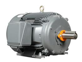
IronHorse MTCP2 premium efficiency AC induction motor, general purpose, inverter rated and severe duty, 100hp, 3-phase, 230/460 VAC, suitable for 208 VAC at 60 Hz, 1800rpm, TEFC, NEMA 405T frame, cast iron, rigid base mount.
