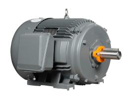
IronHorse MTCP2 premium efficiency AC induction motor, general purpose, inverter rated and severe duty, 60hp, 3-phase, 230/460 VAC, suitable for 208 VAC at 60 Hz, 1800rpm, TEFC, NEMA 364T frame, cast iron, rigid base mount.
