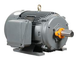
IronHorse MTCP2 premium efficiency AC induction motor, general purpose, inverter rated and severe duty, 50hp, 3-phase, 230/460 VAC, suitable for 208 VAC at 60 Hz, 1800rpm, TEFC, NEMA 326T frame, cast iron, rigid base mount.
