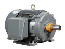
IronHorse MTCP2 premium efficiency AC induction motor, general purpose, inverter rated and severe duty, 40hp, 3-phase, 230/460 VAC, suitable for 208 VAC at 60 Hz, 1800rpm, TEFC, NEMA 324T frame, cast iron, rigid base mount.
