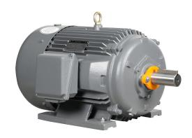
IronHorse MTCP2 premium efficiency AC induction motor, general purpose, inverter rated and severe duty, 30hp, 3-phase, 230/460 VAC, suitable for 208 VAC at 60 Hz, 1800rpm, TEFC, NEMA 286T frame, cast iron, rigid base mount.
