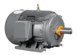
IronHorse MTCP2 premium efficiency AC induction motor, general purpose, inverter rated and severe duty, 25hp, 3-phase, 230/460 VAC, suitable for 208 VAC at 60 Hz, 1800rpm, TEFC, NEMA 284T frame, cast iron, rigid base mount.
