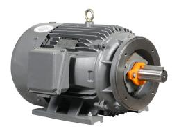
IronHorse MTCP2 premium efficiency AC induction motor, general purpose, inverter rated and severe duty, 25hp, 3-phase, 230/460 VAC, suitable for 208 VAC at 60 Hz, 1800rpm, TEFC, NEMA 284TC frame, cast iron, C-face/rigid base mount.
