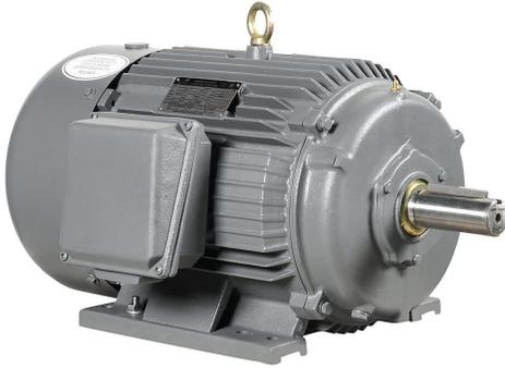
IronHorse MTCP2 premium efficiency AC induction motor, general purpose, inverter rated and severe duty, 20hp, 3-phase, 230/460 VAC, suitable for 208 VAC at 60 Hz, 3600rpm, TEFC, NEMA 256T frame, cast iron, rigid base mount.
