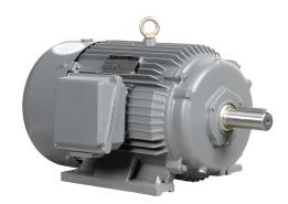
IronHorse MTCP2 premium efficiency AC induction motor, general purpose, inverter rated and hazardous location, 20hp, 3-phase, 230/460 VAC, suitable for 208 VAC at 60 Hz, 1800rpm, TEFC, 256T frame, cast iron, rigid base mount.
