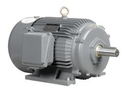
IronHorse MTCP2 premium efficiency AC induction motor, general purpose, inverter rated and severe duty, 20hp, 3-phase, 230/460 VAC, suitable for 208 VAC at 60 Hz, 1800rpm, TEFC, NEMA 256T frame, cast iron, rigid base mount.
