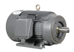
IronHorse MTCP2 premium efficiency AC induction motor, general purpose, inverter rated and severe duty, 20hp, 3-phase, 230/460 VAC, suitable for 208 VAC at 60 Hz, 1800rpm, TEFC, NEMA 256TC frame, cast iron, C-face/rigid base mount.
