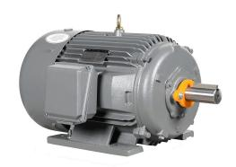
IronHorse MTCP2 premium efficiency AC induction motor, general purpose, inverter rated and severe duty, 20hp, 3-phase, 230/460 VAC, suitable for 208 VAC at 60 Hz, 1200rpm, TEFC, NEMA 286T frame, cast iron, rigid base mount.
