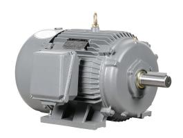
IronHorse MTCP2 premium efficiency AC induction motor, general purpose, inverter rated and severe duty, 15hp, 3-phase, 230/460 VAC, suitable for 208 VAC at 60 Hz, 1800rpm, TEFC, NEMA 254T frame, cast iron, rigid base mount.
