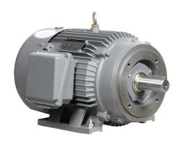
IronHorse MTCP2 premium efficiency AC induction motor, general purpose, inverter rated and severe duty, 15hp, 3-phase, 230/460 VAC, suitable for 208 VAC at 60 Hz, 1800rpm, TEFC, NEMA 254TC frame, cast iron, C-face/rigid base mount.
