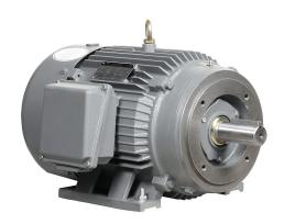
IronHorse MTCP2 premium efficiency AC induction motor, general purpose, inverter rated and hazardous location, 15hp, 3-phase, 230/460 VAC, suitable for 208 VAC at 60 Hz, 1800rpm, TEFC, 254TC frame, cast iron, C-face/rigid base mount.
