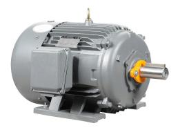
IronHorse MTCP2 premium efficiency AC induction motor, general purpose, inverter rated and severe duty, 15hp, 3-phase, 230/460 VAC, suitable for 208 VAC at 60 Hz, 1200rpm, TEFC, NEMA 284T frame, cast iron, rigid base mount.
