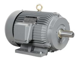
IronHorse MTCP2 premium efficiency AC induction motor, general purpose, inverter rated and hazardous location, 10hp, 3-phase, 230/460 VAC, suitable for 208 VAC at 60 Hz, 3600rpm, TEFC, 215T frame, cast iron, rigid base mount.
