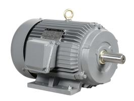
IronHorse MTCP2 premium efficiency AC induction motor, general purpose, inverter rated and severe duty, 10hp, 3-phase, 230/460 VAC, suitable for 208 VAC at 60 Hz, 1800rpm, TEFC, NEMA 215T frame, cast iron, rigid base mount.
