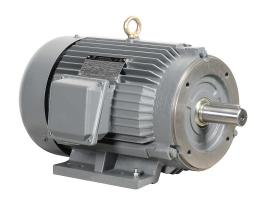
IronHorse MTCP2 premium efficiency AC induction motor, general purpose, inverter rated and severe duty, 10hp, 3-phase, 230/460 VAC, suitable for 208 VAC at 60 Hz, 1800rpm, TEFC, 215TC frame, cast iron, C-face/rigid base mount.
