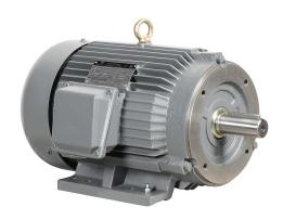
IronHorse MTCP2 premium efficiency AC induction motor, general purpose, inverter rated and hazardous location, 10hp, 3-phase, 230/460 VAC, suitable for 208 VAC at 60 Hz, 1800rpm, TEFC, 215TC frame, cast iron, C-face/rigid base mount.
