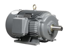
IronHorse MTCP2 premium efficiency AC induction motor, general purpose, inverter rated and severe duty, 10hp, 3-phase, 230/460 VAC, suitable for 208 VAC at 60 Hz, 1200rpm, TEFC, 256T frame, cast iron, rigid base mount.
