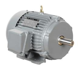
IronHorse MTCP2 premium efficiency AC induction motor, general purpose, inverter rated and severe duty, 5hp, 3-phase, 230/460 VAC, suitable for 208 VAC at 60 Hz, 3600rpm, TEFC, NEMA 184T frame, cast iron, rigid base mount.
