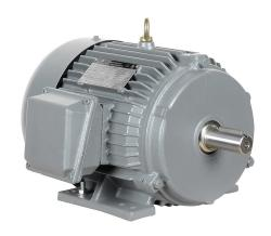
IronHorse MTCP2 premium efficiency AC induction motor, general purpose, inverter rated and severe duty, 5hp, 3-phase, 230/460 VAC, suitable for 208 VAC at 60 Hz, 1800rpm, TEFC, NEMA 184T frame, cast iron, rigid base mount.
