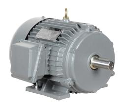
IronHorse MTCP2 premium efficiency AC induction motor, general purpose, inverter rated and hazardous location, 5hp, 3-phase, 230/460 VAC, suitable for 208 VAC at 60 Hz, 1800rpm, TEFC, 184T frame, cast iron, rigid base mount.
