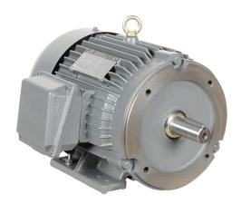
IronHorse MTCP2 premium efficiency AC induction motor, general purpose, inverter rated and severe duty, 5hp, 3-phase, 230/460 VAC, suitable for 208 VAC at 60 Hz, 1800rpm, TEFC, NEMA 184TC frame, cast iron, C-face/rigid base mount.
