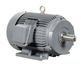
IronHorse MTCP2 premium efficiency AC induction motor, general purpose, inverter rated and severe duty, 5hp, 3-phase, 230/460 VAC, suitable for 208 VAC at 60 Hz, 1200rpm, TEFC, NEMA 215T frame, cast iron, rigid base mount.
