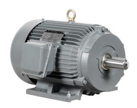
IronHorse MTCP2 premium efficiency AC induction motor, general purpose, inverter rated and hazardous location, 5hp, 3-phase, 230/460 VAC, suitable for 208 VAC at 60 Hz, 1200rpm, TEFC, 215T frame, cast iron, rigid base mount.
