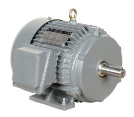
IronHorse MTCP2 premium efficiency AC induction motor, general purpose, inverter rated and severe duty, 3hp, 3-phase, 230/460 VAC, suitable for 208 VAC at 60 Hz, 3600rpm, TEFC, NEMA 182T frame, cast iron, rigid base mount.
