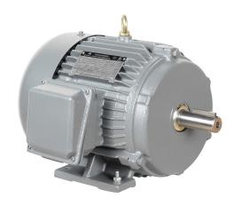
IronHorse MTCP2 premium efficiency AC induction motor, general purpose, inverter rated and severe duty, 3hp, 3-phase, 230/460 VAC, suitable for 208 VAC at 60 Hz, 1800rpm, TEFC, NEMA 182T frame, cast iron, rigid base mount.
