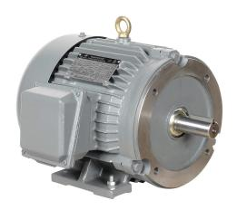
IronHorse MTCP2 premium efficiency AC induction motor, general purpose, inverter rated and hazardous location, 3hp, 3-phase, 230/460 VAC, suitable for 208 VAC at 60 Hz, 1800rpm, TEFC, 182TC frame, cast iron, C-face/rigid base mount.
