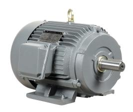
IronHorse MTCP2 premium efficiency AC induction motor, general purpose, inverter rated and severe duty, 3hp, 3-phase, 230/460 VAC, suitable for 208 VAC at 60 Hz, 1200rpm, TEFC, NEMA 213T frame, cast iron, rigid base mount.
