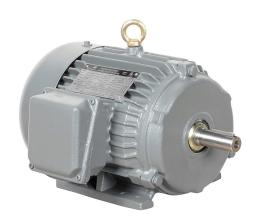
IronHorse MTCP2 premium efficiency AC induction motor, general purpose, inverter rated and severe duty, 2hp, 3-phase, 230/460 VAC, suitable for 208 VAC at 60 Hz, 3600rpm, TEFC, NEMA 145T frame, cast iron, rigid base mount.
