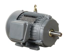
IronHorse MTCP2 premium efficiency AC induction motor, general purpose, inverter rated and severe duty, 2hp, 3-phase, 230/460 VAC, suitable for 208 VAC at 60 Hz, 1800rpm, TEFC, NEMA 145T frame, cast iron, rigid base mount.
