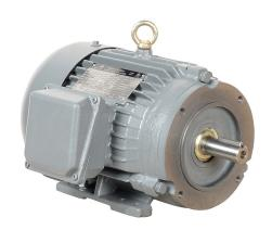
IronHorse MTCP2 premium efficiency AC induction motor, general purpose, inverter rated and severe duty, 2hp, 3-phase, 230/460 VAC, suitable for 208 VAC at 60 Hz, 1800rpm, TEFC, NEMA 145TC frame, cast iron, C-face/rigid base mount.
