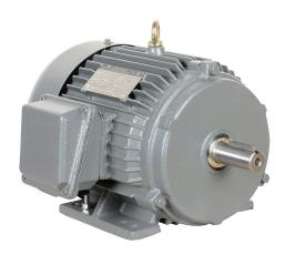
IronHorse MTCP2 premium efficiency AC induction motor, general purpose, inverter rated and hazardous location, 2hp, 3-phase, 230/460 VAC, suitable for 208 VAC at 60 Hz, 1200rpm, TEFC, 184T frame, cast iron, rigid base mount.
