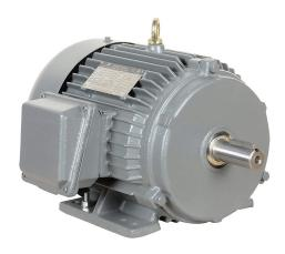
IronHorse MTCP2 premium efficiency AC induction motor, general purpose, inverter rated and severe duty, 2hp, 3-phase, 230/460 VAC, suitable for 208 VAC at 60 Hz, 1200rpm, TEFC, NEMA 184T frame, cast iron, rigid base mount.
