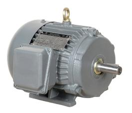
IronHorse MTCP2 premium efficiency AC induction motor, general purpose, inverter rated and severe duty, 1hp, 3-phase, 230/460 VAC, suitable for 208 VAC at 60 Hz, 1800rpm, TEFC, NEMA 143T frame, cast iron, rigid base mount.
