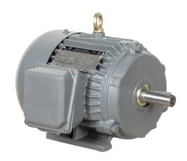
IronHorse MTCP2 premium efficiency AC induction motor, general purpose, inverter rated and hazardous location, 1hp, 3-phase, 230/460 VAC, suitable for 208 VAC at 60 Hz, 1800rpm, TEFC, 143T frame, cast iron, rigid base mount.
