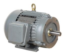
IronHorse MTCP2 premium efficiency AC induction motor, general purpose, inverter rated and severe duty, 1hp, 3-phase, 230/460 VAC, suitable for 208 VAC at 60 Hz, 1800rpm, TEFC, NEMA 143TC frame, cast iron, C-face/rigid base mount.
