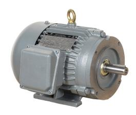
IronHorse MTCP2 premium efficiency AC induction motor, general purpose, inverter rated and hazardous location, 1hp, 3-phase, 230/460 VAC, suitable for 208 VAC at 60 Hz, 1800rpm, TEFC, 143TC frame, cast iron, C-face/rigid base mount.
