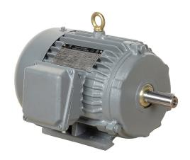
IronHorse MTCP2 premium efficiency AC induction motor, general purpose, inverter rated and severe duty, 1hp, 3-phase, 230/460 VAC, suitable for 208 VAC at 60 Hz, 1200rpm, TEFC, NEMA 145T frame, cast iron, rigid base mount.
