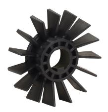
IronHorse MTCP2 series main cooling fan, replacement. For use with 4-pole and 6-pole 213 and 215 frame IronHorse premium efficiency MTCP2 series motors. Not compatible with MTC or MTCP series motors.
