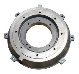
IronHorse C-flange, replacement. For use with 449T frame IronHorse premium efficiency MTCP2 series motors. Mounting hardware included. Replaces drive end bell, field install. Not compatible with MTC or MTCP series motors.
