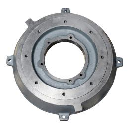
IronHorse C-flange, replacement. For use with 447T frame IronHorse premium efficiency MTCP2 series motors. Mounting hardware included. Replaces drive end bell, field install. Not compatible with MTC or MTCP series motors.
